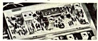
Advanced FM Frontend: Three low-noise MOS FETs are employed for the two RF stages and the mixer stage. Combined with a 4-gang variable capacitor, they ensure an exceptional sensitivity figure of 1.8 µV (IHF), and result in a substantially improved intermodulation distortion factor as well as enhanced image and S/N ratios. Exceptionally steady hi-fi FM stereo reception even in remote areas is now a reality
